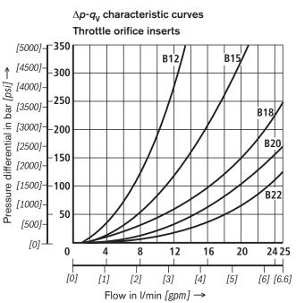
Power limits (measured with HLP46,  $\vartheta_{\text{oil}}$  (v = 190 SUS) = 40 °C ± 5 °C [104 °F ± 9 °F])
