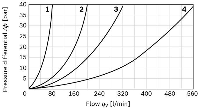
▼ **Pressure differential  $\Delta p$  in relation to flow  $q_v$ , measured via the check valve: A  $\rightarrow$  B**
