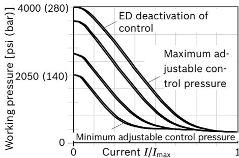
► Hysteresis static current-pressure characteristic curve < 45 psi (3 bar).
