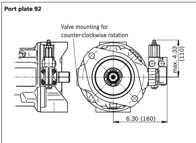
▼ **DRG – Pressure controller, remote controlled**
