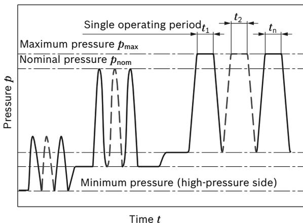
Total operating period =  $t_1 + t_2 + \dots + t_n$
