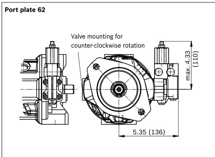
▼ **DRG – Pressure controller, remote controlled**
