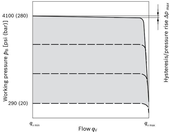
Characteristic curve valid at  $n_1 = 1500$  rpm and  $\theta_{\text{fluid}} = 122$  °F (50 °C).
