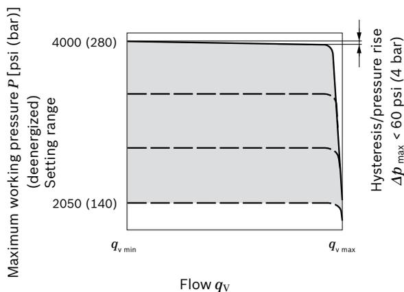
Characteristic curve valid at  $n_1 = 1500$  rpm and  $\theta_{\text{fluid}} = 122$  °F (50 °C).
