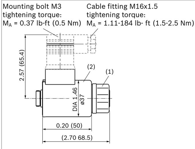
The seal ring in the cable fitting is suitable for lines of diameter 0.18 in to 0.39 in (4.5 mm to 10 mm).
