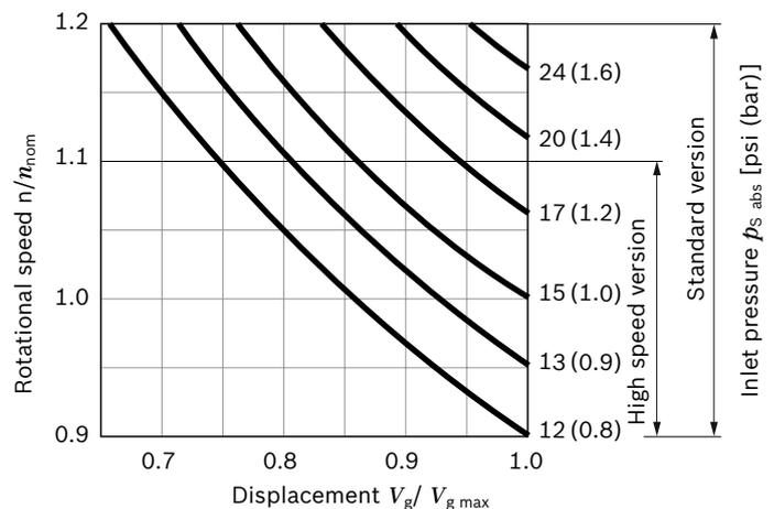
During continuous operation in overspeed over  $n_{nom}$ , a reduction in operational service life is to be expected due to cavitation erosion.
